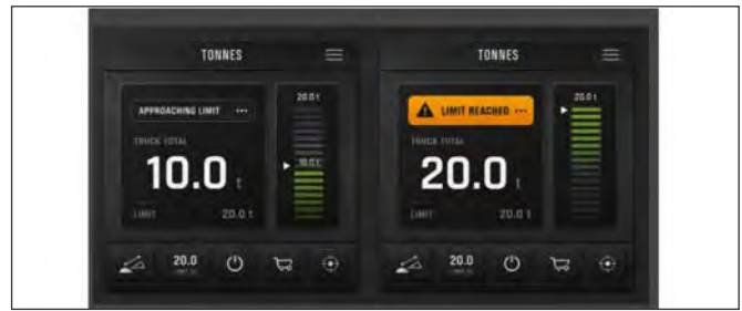
Stage 5: State threshold system Clarified safe, approaching, and limit states through segmented progression.
