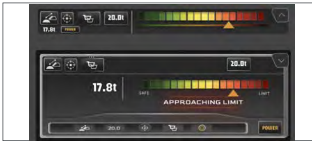
Stage 4: Condensed horizontal Moved payload communication into a compact lateral scan path and reduced vertical demand.
